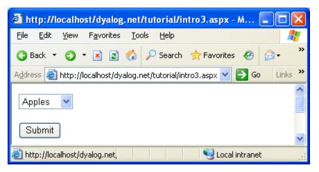
In this example, the page is processed by a POST back caused by pressing the Submit button. As it stands, changing the selection in the list object does not cause the text in the out object to be changed; you have to press the Submit button first.
