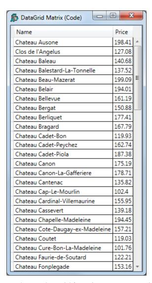
In order to apply special formatting to one or more columns, it is necessary to set the AutoGenerateColumns property to 0, and to generate the columns programatically as is shown in the second version of the function, GridCode.
