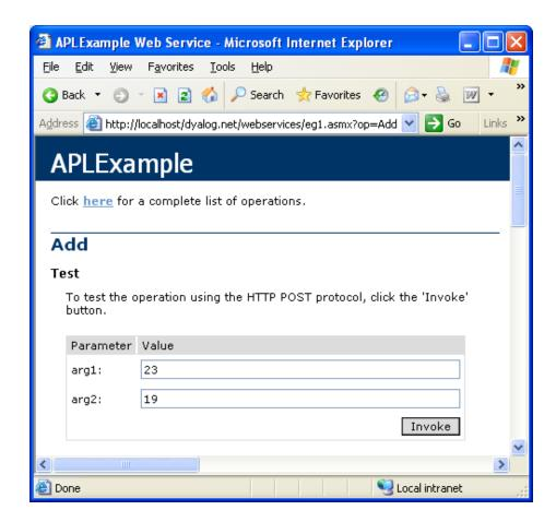
The following screen shot shows the result of entering the values 23 and 19 into the form fields and then pressing the Invoke button.
