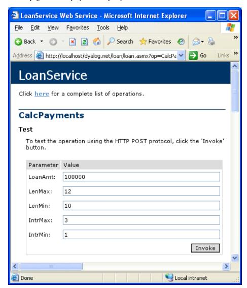
To test the CalcPayments method, you can enter numbers into the form fields in this page, as shown in the screen shot above, and then press the *Invoke* button. The result of the method is then displayed in a separate window as illustrated below.
