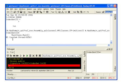
Notice too that IndexGen has been started on APL thread 1 which, in this case, is associated with system thread 4056. If the client application were to call IndexGen on multiple system threads, this would be reflected by multiple APL threads in the workspace. This topic is discussed in further detail below.
