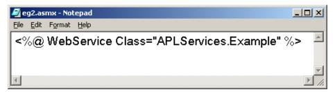
Given this instruction, ASP.NET will locate the APLServices. Example Web Service by searching the bin sub-directory for assemblies. Therefore, to make this work, we have only to create a .NET assembly in samples\asp.net\bin. The assembly should contain a .NET Namespace named APLServices, which in turn defines a class named Example.
