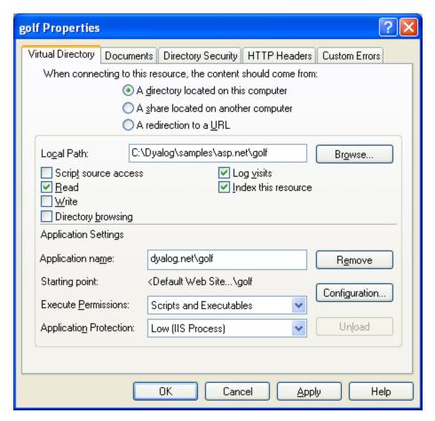
Note that the *Application Protection* entry dictates whether your application is loaded into the IIS process (Low), a shared DLLHost task (Medium) or its own DLLHost task (High). The last choice isolates your application from all other IIS applications, and is the safest option.
