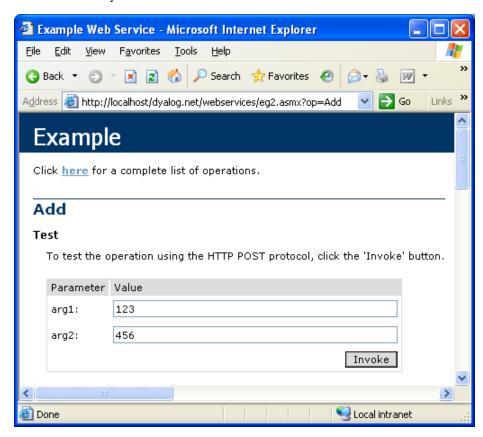
If you enter the numbers 123 and 456 in the fields provided, then press *Invoke*, the method will be called and the result displayed as shown below.
