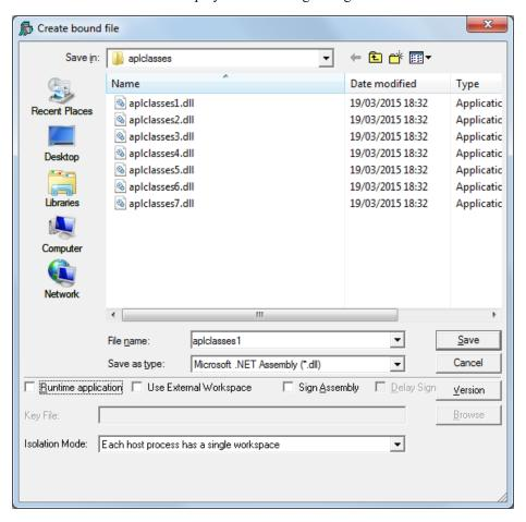
This gives you the opportunity to change the name or path of the assembly. The *Runtime application* checkbox allows you to choose to which if the two versions of the Dyalog APL dynamic link library the assembly will be bound. The Isolation Mode Combo box allows you to choose which Isolation Mode you require. See the *User Guide* for further details.
